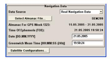
The **Navigation Data** menu section is where the data source for navigation information is selected and the data indicated (in case of real navigation data).
