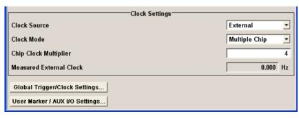
The Clock Settings section is where the clock source is selected and - in the case of an external source - the clock type. The Global Trigger/Clock Settings button leads to a submenu for general trigger and clock settings.
